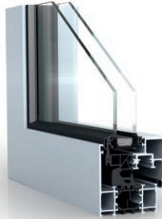
The option "Concealed Sash" in the aluminium window system WICLINE evo features a special glazing bead fixed directly in the thermal break zone. As a result the system achieves an extremely slim frame elevation, superior thermal insulation values and a sleek profile design from outside. The improved ratio between frame and glazing surfaces leads to very good  $U_w$  values, increased light transmissions and panoramic views.
