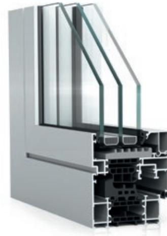
With 75 mm profile depth, WICLINE 75 evo features the highest thermal insulation properties and structural characteristics. With its superior technical performance this aluminium window is at-tuned to all architectural requirements of the future. In Switzerland WICLINE 75 evo has been the first metal window to be certified as Minergie-P module window.
