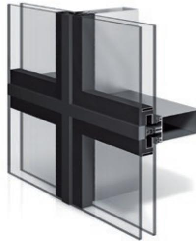
A characteristic feature of WICTEC 50SG structural glazing curtain wall is the flush design with slim silicone joints between the glass panes. The system offers all-glass technology both for vertical curtain walls and sloped roof glazing. Based on the standard WICTEC 50 stick system these options can be realised with simplified and economic processing and assembly, while assuring a high level of quality.
